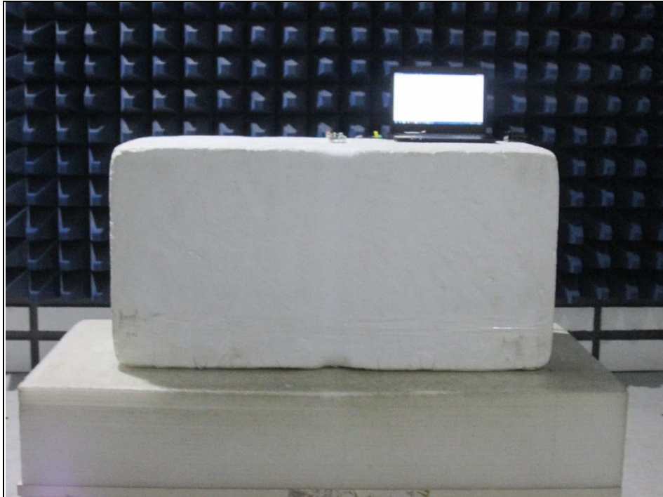
Radiated Emission Test above 1GHz
