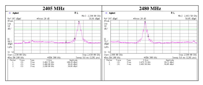
\* Final result of band edge was measured as radiated spurious emission. Refer to Radiated Spurious Emission's pages.
