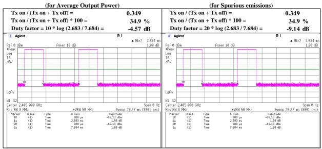
\* When testing (Average output power, Spurious emissions), it measured by the signal of duty 100 %, and it was corrected measuring value the duty of normal operation.
