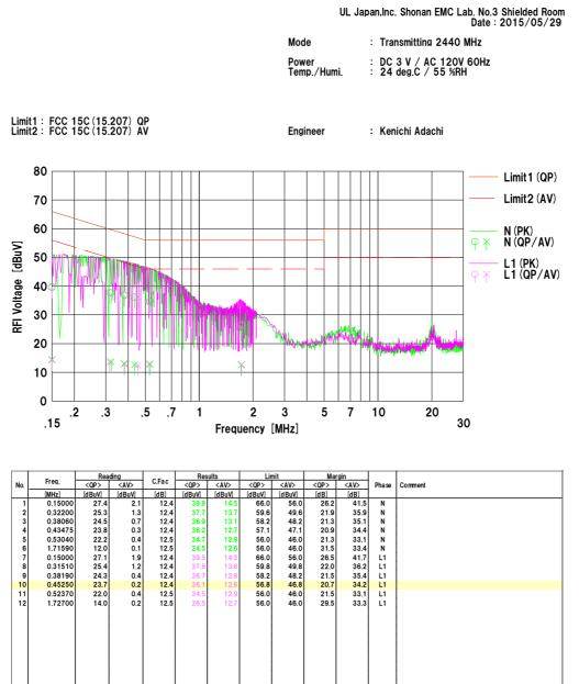
Calculation:Result [dBuV] =Reading [dBuV] +C.Fac (LISN+Cable+ATT) [dB] LISN: SLS-05
