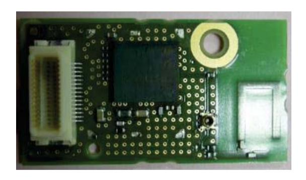
The antenna connector is used for pre-shipping inspection only.
