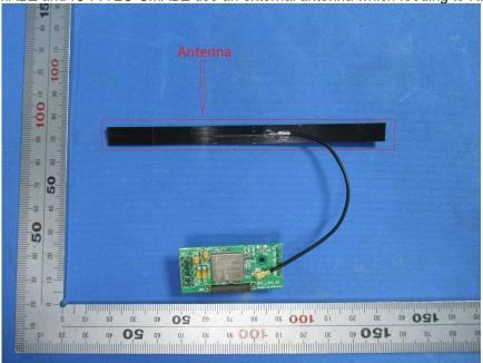
We apply for Limited Modular Transmitter Approval because the module doesn't fulfil the antenna condition as described above. A PIFA antenna (ANT-TE-LTFR-225 from KTM, gain=2.0dBi) was adopted to perform the radiated tests of Limited Modular Transmitter Approval.
