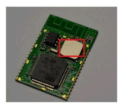
FCCID is marked on AAD metalcase by laser
