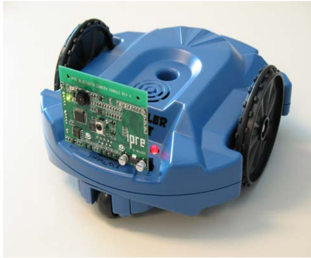
Fluke Robot upgrade module installed on a Parallax scribbler robot.
