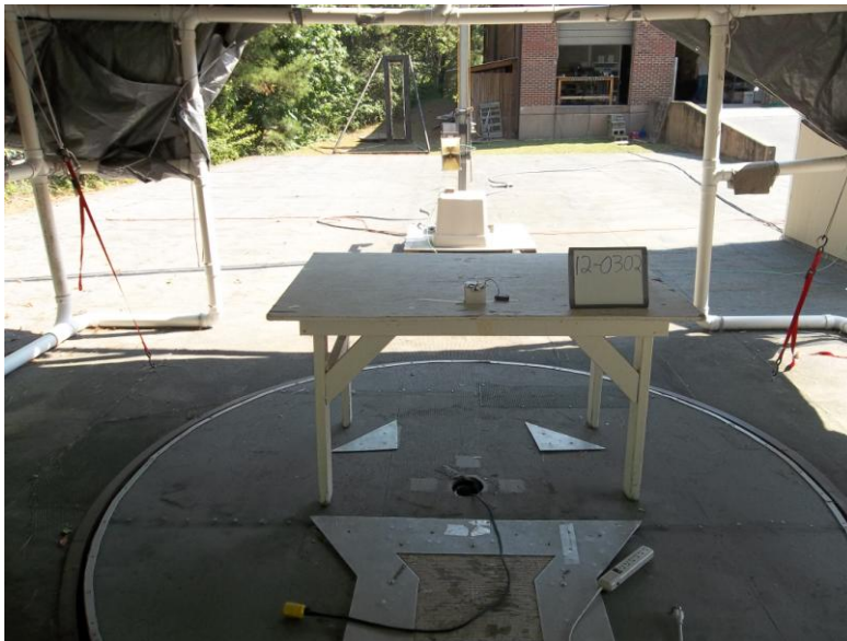
Rear View Radiated emissions Test setup.
