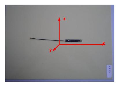
FXP831 on Baxter device to indicate the testing coordinate
