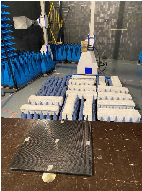
Test setup in anechoic chamber – Frequency >1GHz
