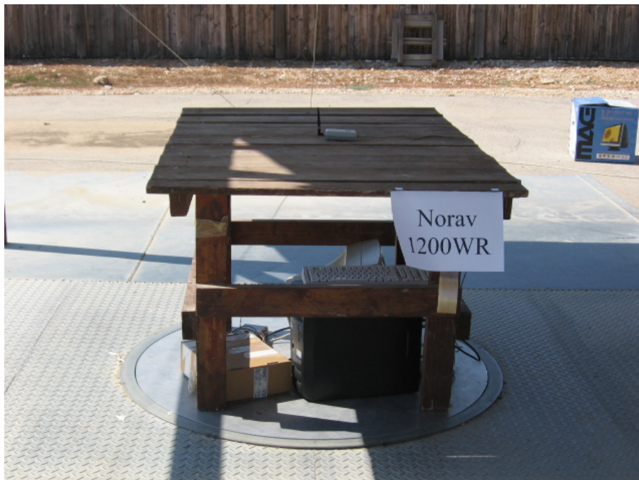
Figure 10. Radiated Emission Test Side
