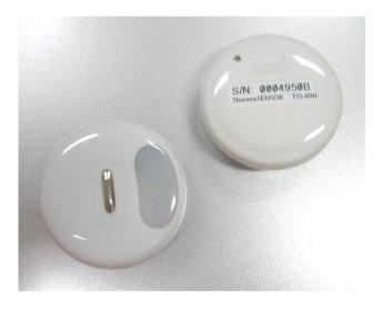
Every 30 seconds, the sensor will take a temperature measurement and transmits the measured temperature to the SMN-800/900 SmartNODE.
