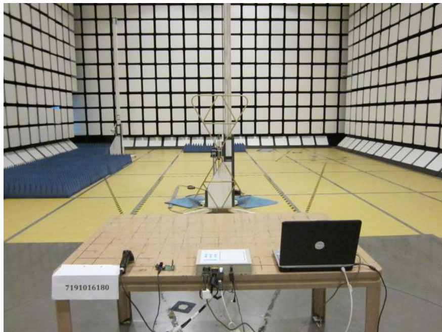
Radiated Emissions Test Setup (Rear View)
