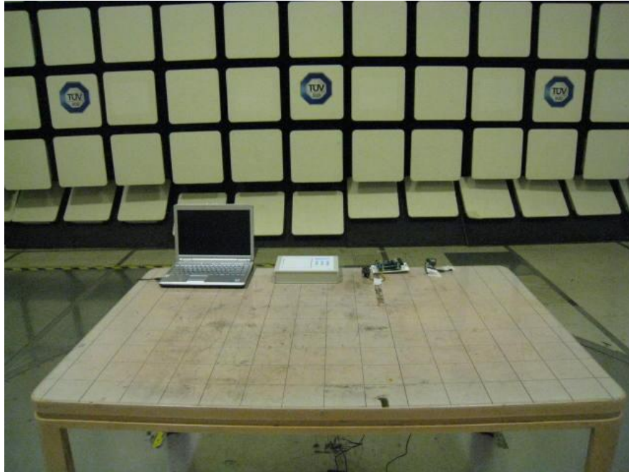
Radiated Emissions Test Setup (Front View)
