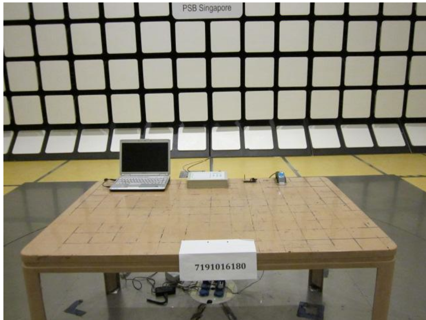
Radiated Emissions Test Setup (Front View)
