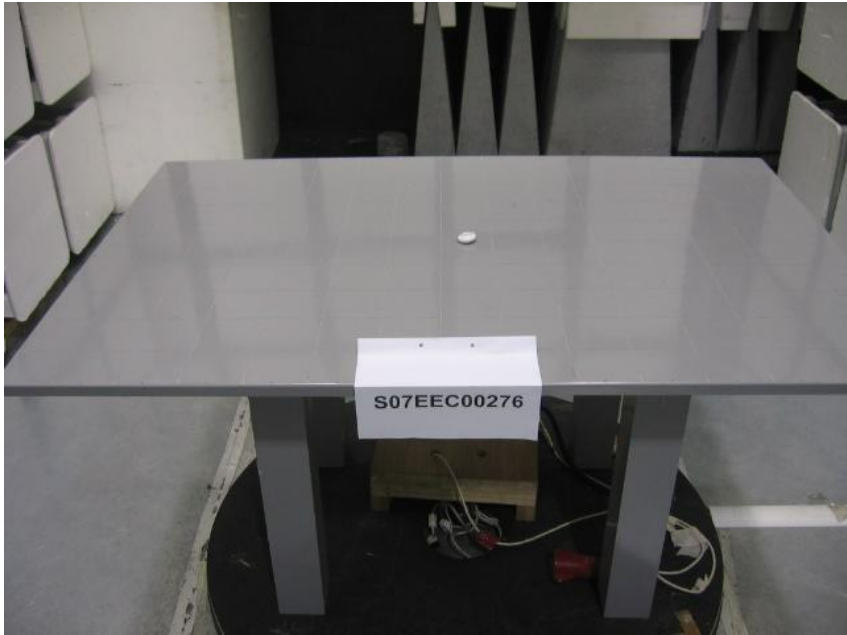
Radiated Emissions Test Setup (Front View)
