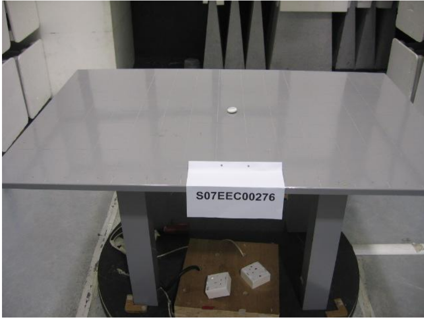
Radiated Emissions Test Setup (Rear View)
