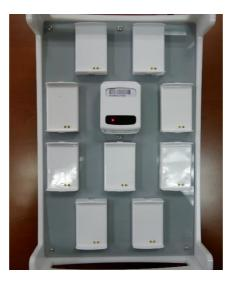
When the tag is fully charged the Green LED will light up as shown below.
