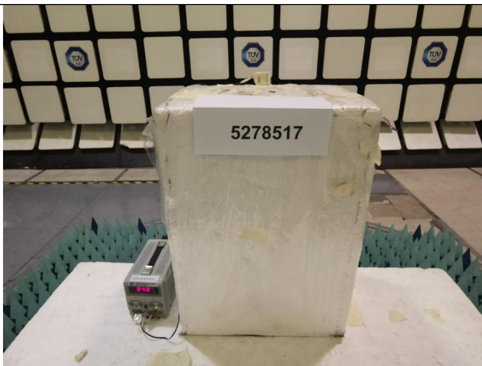
Radiated Emissions (Spurious Emissions Inclusive Restricted Bands Requirement) Test Setup (Front View)
