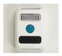
When the STG-873W passes by a LF exciter (typically installed at key chokepoints or egress points) it will receive a location ID transmitted by the exciter. The tag will transmit a WiFi signal to update tag status and tag location to the location tracking system.
