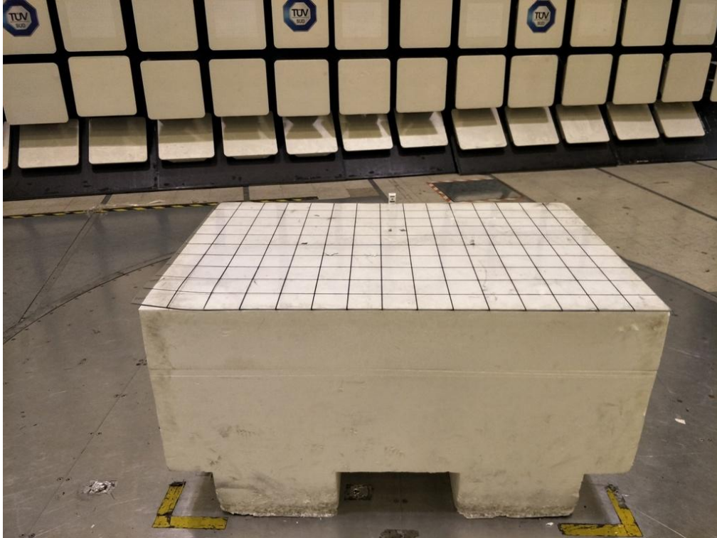
Radiated Emissions Test Setup (Front View)
