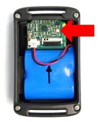
CAUTION: Press button to reset tag to ensure proper power up.
