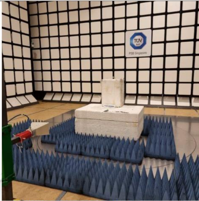
Radiated Emissions (Spurious Emissions Inclusive Restricted Bands Requirement) Test Setup (Front View)
