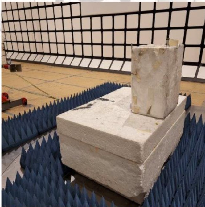
Radiated Emissions (Spurious Emissions Inclusive Restricted Bands Requirement) Test Setup (Rear View)
