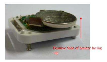
5. Lastly, tighten the casings with the 4 screws
