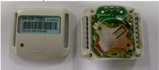
4. To replace a new battery, slide the battery into the battery holder from the position as shown on picture below. Make sure the positive side of battery is facing up.
