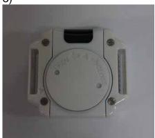
Adjust the battery cover as shown above (*triangle pointing at about 1'o clock*) so that >90% of the thickness of the cover is inserted into the casing (body).
