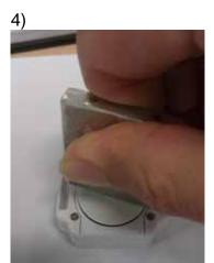
Press a little bit and turning clockwise for tightening. (*Approximately 10 degree, there is a stopper so won't overturn*).
