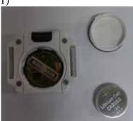
Prepare a CR2050 coin cell battery and a battery cover as shown above
