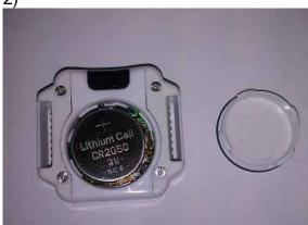
Place the coin-cell battery with positive terminal (+) face outwards.
