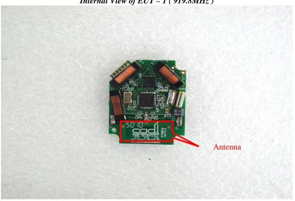
Internal View of EUT - 2(919.8MHz)
