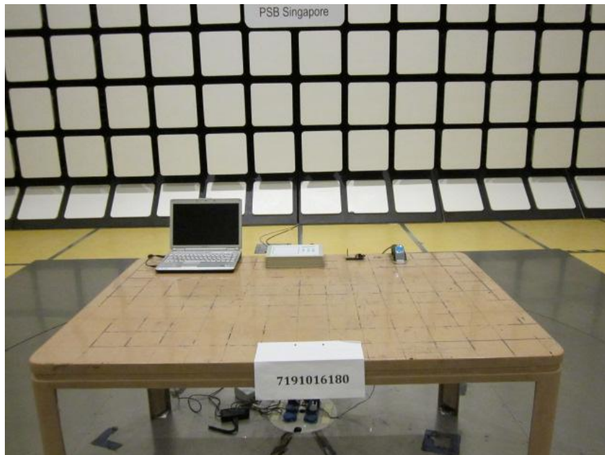
Radiated Emissions Test Setup (Front View)
