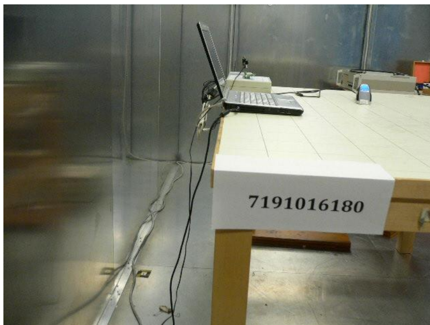
Conducted Emissions Test Setup (Rear View)
