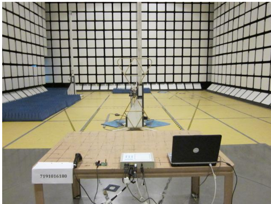
Radiated Emissions Test Setup (Rear View)
