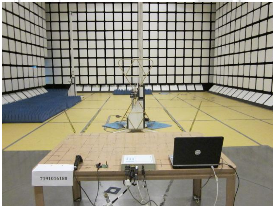
Radiated Emissions Test Setup (Rear View)
