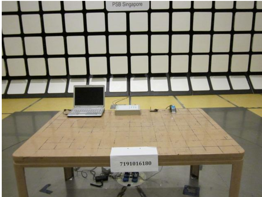
Radiated Emissions Test Setup (Front View)
