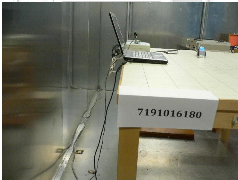
Conducted Emissions Test Setup (Rear View)
