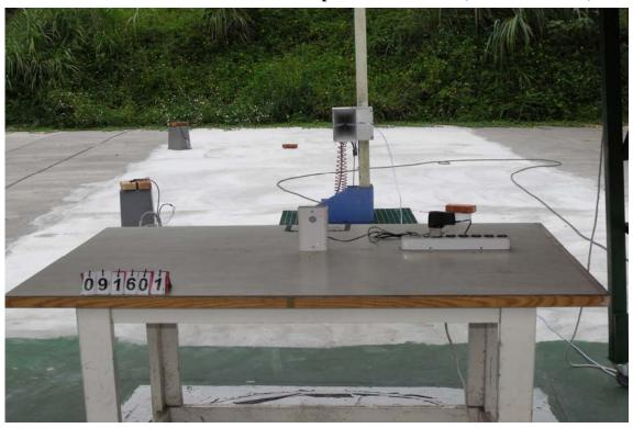
Vertical Polarization and the EUT place to the X axis (1GHz to 10GHz)
