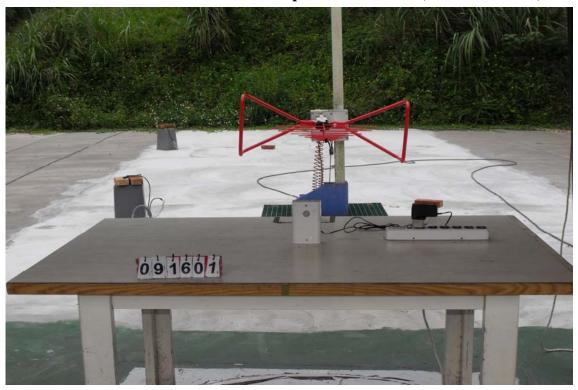
Vertical Polarization and the EUT place to the X axis (30MHz to 1GHz)
