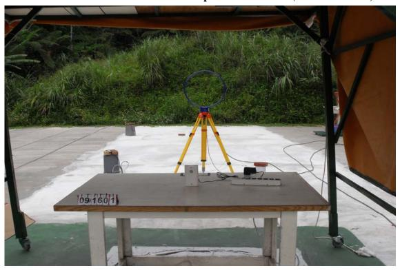
Vertical Polarization and the EUT place to the X axis (9kHz to 30MHz)
