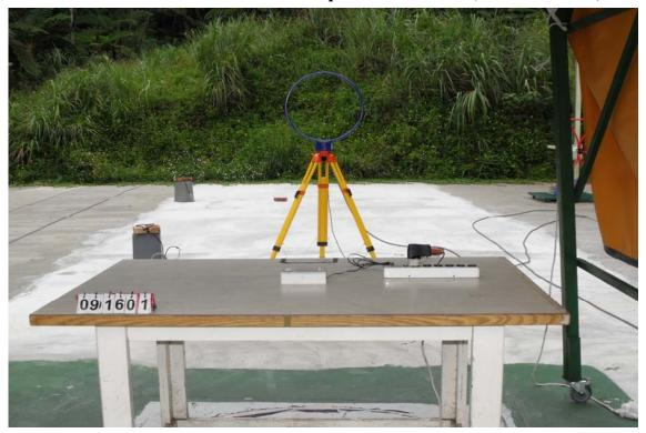
Horizontal Polarization and the EUT place to the Y axis (9kHz to 30MHz)
