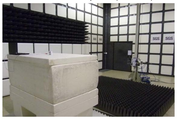
Radiated Emission Set up Photos (Front View)
