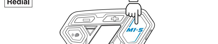
When the device is on, short press function button twice, will redial, blue light flashes
