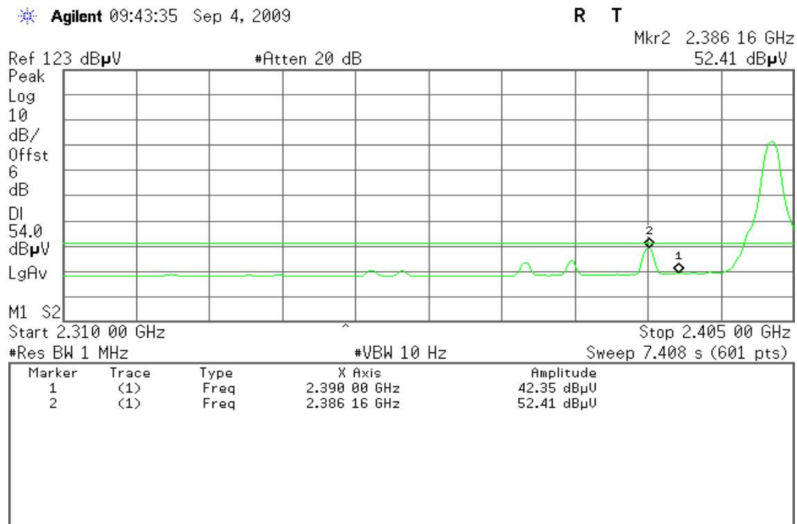
**Band Edges (Bluetooth / CH High)****Detector mode: Peak****Polarity: Vertical**
