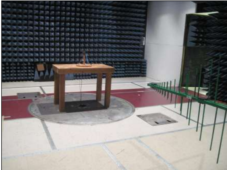
Photograph 3. Radiated Spurious Emissions 30 MHz – 1 GHz, Test Setup
