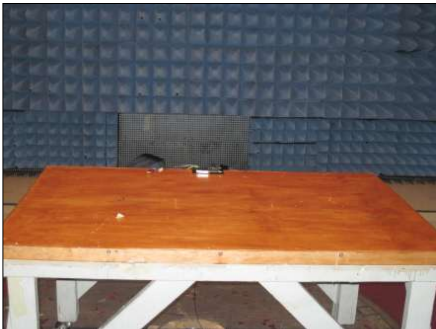
Photograph 2. Radiated Emission, Test Setup
