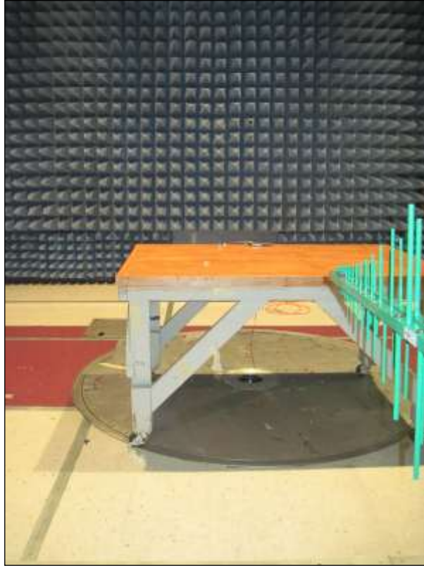
Photograph 1. Radiated Emissions, Test Setup, Antenna View
