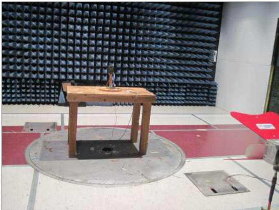
Photograph 4. Radiated Spurious Emissions 1 GHz – 18 GHz, Test Setup
