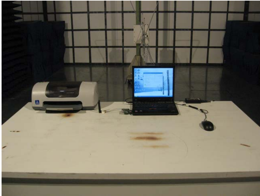
Photo of Radiated Emission Test (Below 1GHz)
