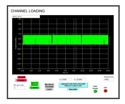
The level of traffic loading on the channel by the EUT is 90.66%
