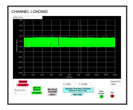
The level of traffic loading on the channel by the EUT is 80.652%
