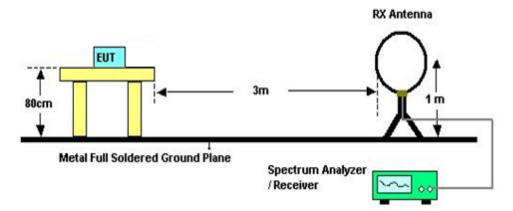
(B) Radiated Emission Test Set-Up Frequency Below 1 GHz
