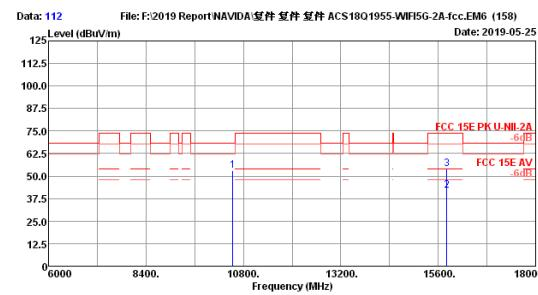
Remarks: 1. Emission Level= Antenna Factor + Cable Loss + Reading
