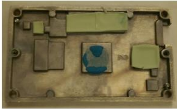
Heat Sink Internal View
