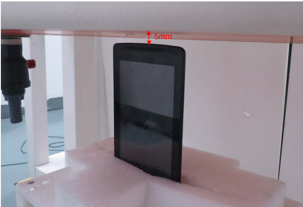
Picture 22: Test Position 5 (Distance 5mm)
