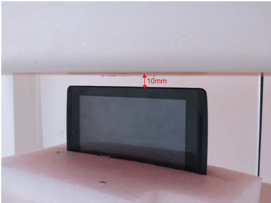
Picture 17: Test Position 3 (Distance 10mm)
