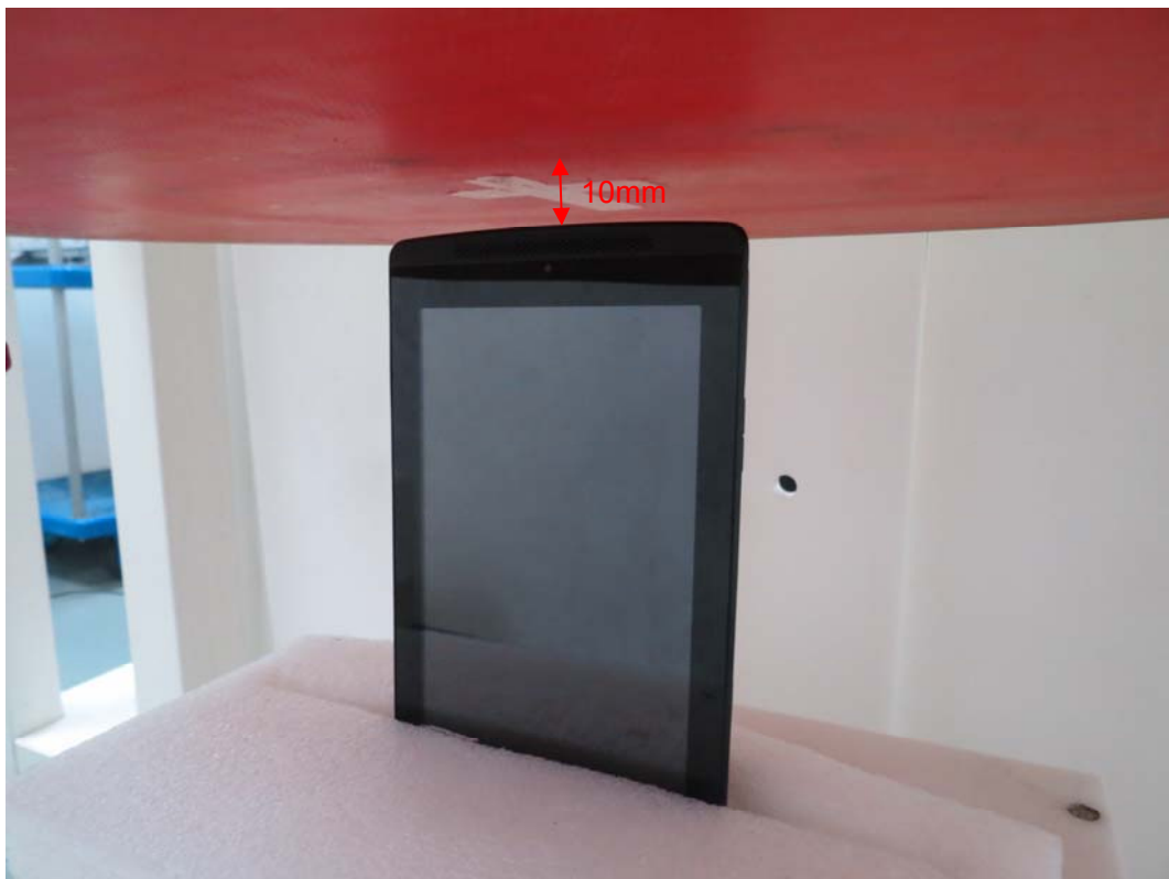
Picture 20: Test Position 4 (Distance 10mm)
