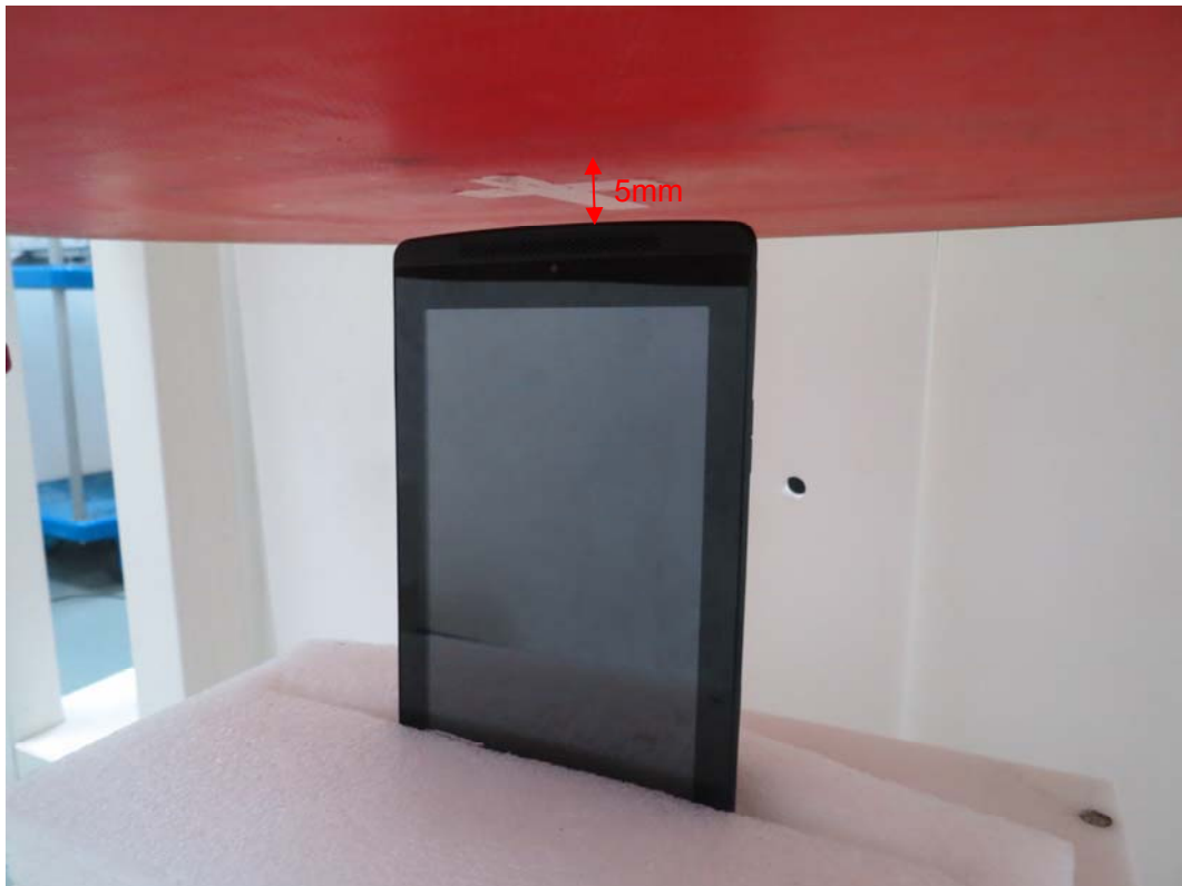
Picture 19: Test Position 4 (Distance 5mm)
