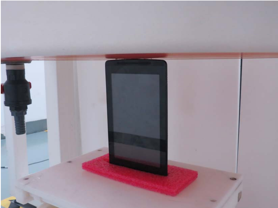
Picture 21: Test Position 5 (Distance 0mm)
