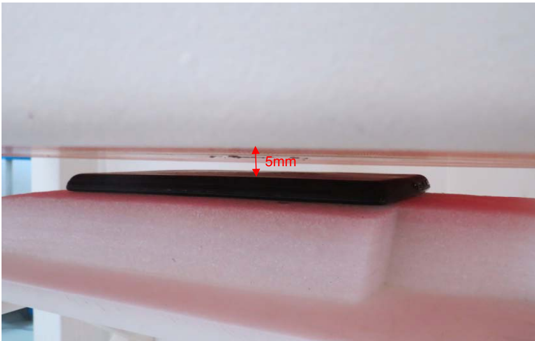
Picture 10: Test position 1 (Distance 5mm)
