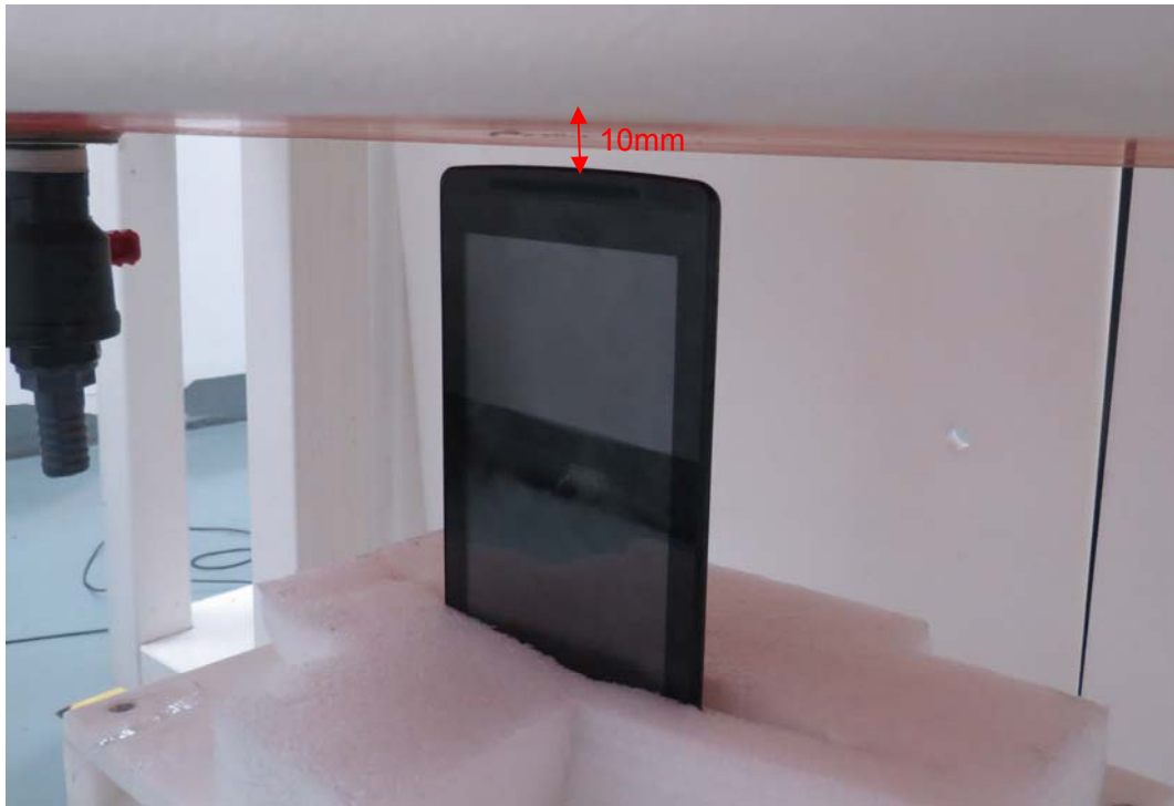
Picture 23: Test Position 5 (Distance 10mm)
