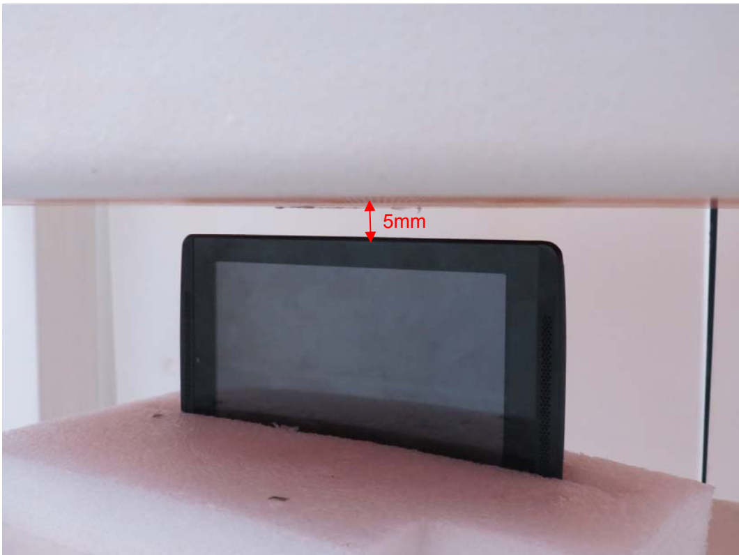
Picture 16: Test Position 3 (Distance 5mm)
