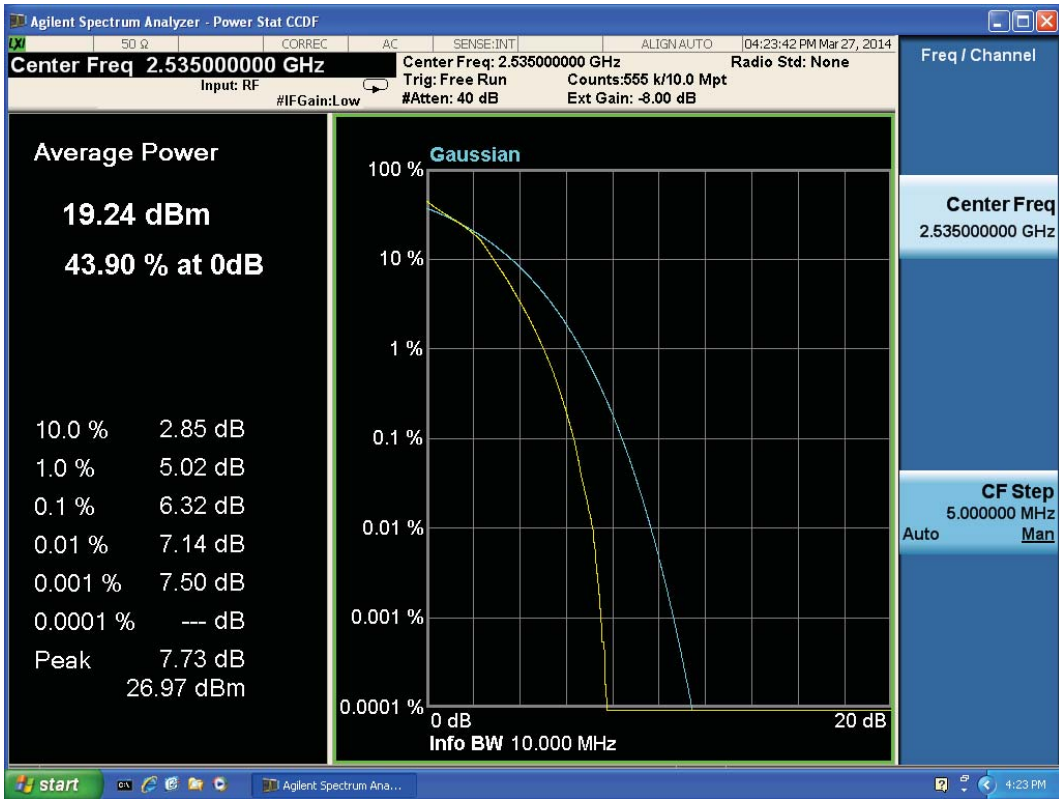
LTE Band 7 16QAM Bandwidth = 10MHz CH21100
