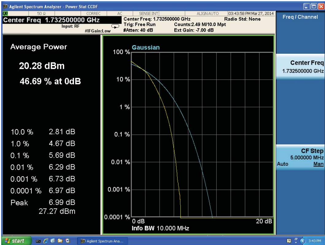
LTE Band 4 16QAM Bandwidth = 10MHz CH20175
