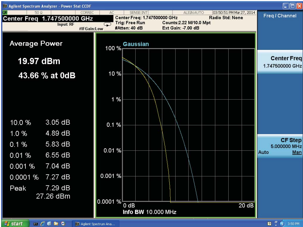
LTE Band 4 16QAM Bandwidth = 15MHz CH20325
