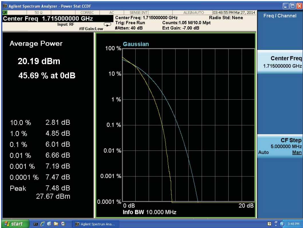
LTE Band 4 16QAM Bandwidth = 10MHz CH20000
