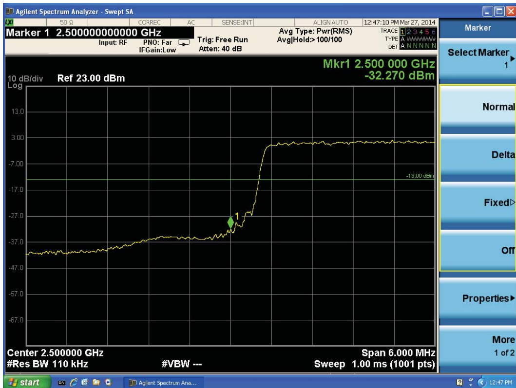
LTE Band 7 16QAM Bandwidth = 10MHz CH20800, RB 50
