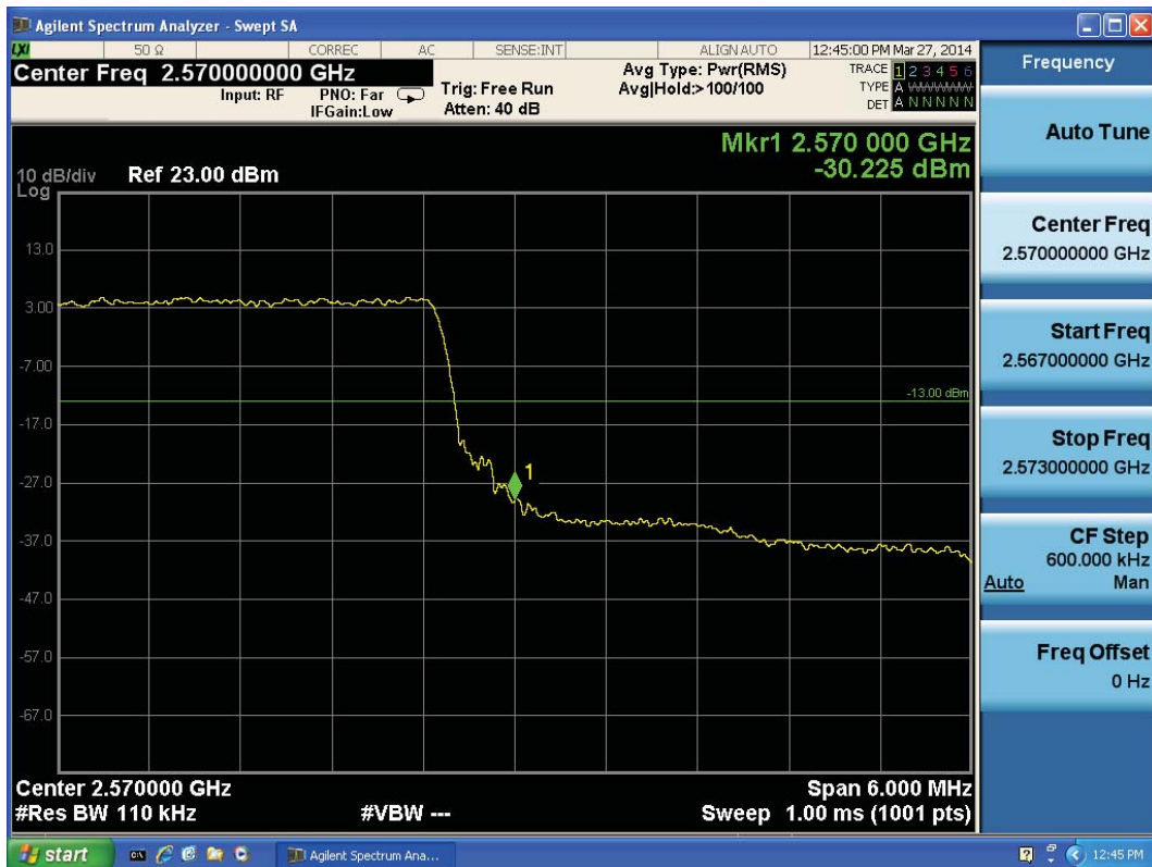
LTE Band 7 16QAM Bandwidth = 10MHz CH21400, RB 25
