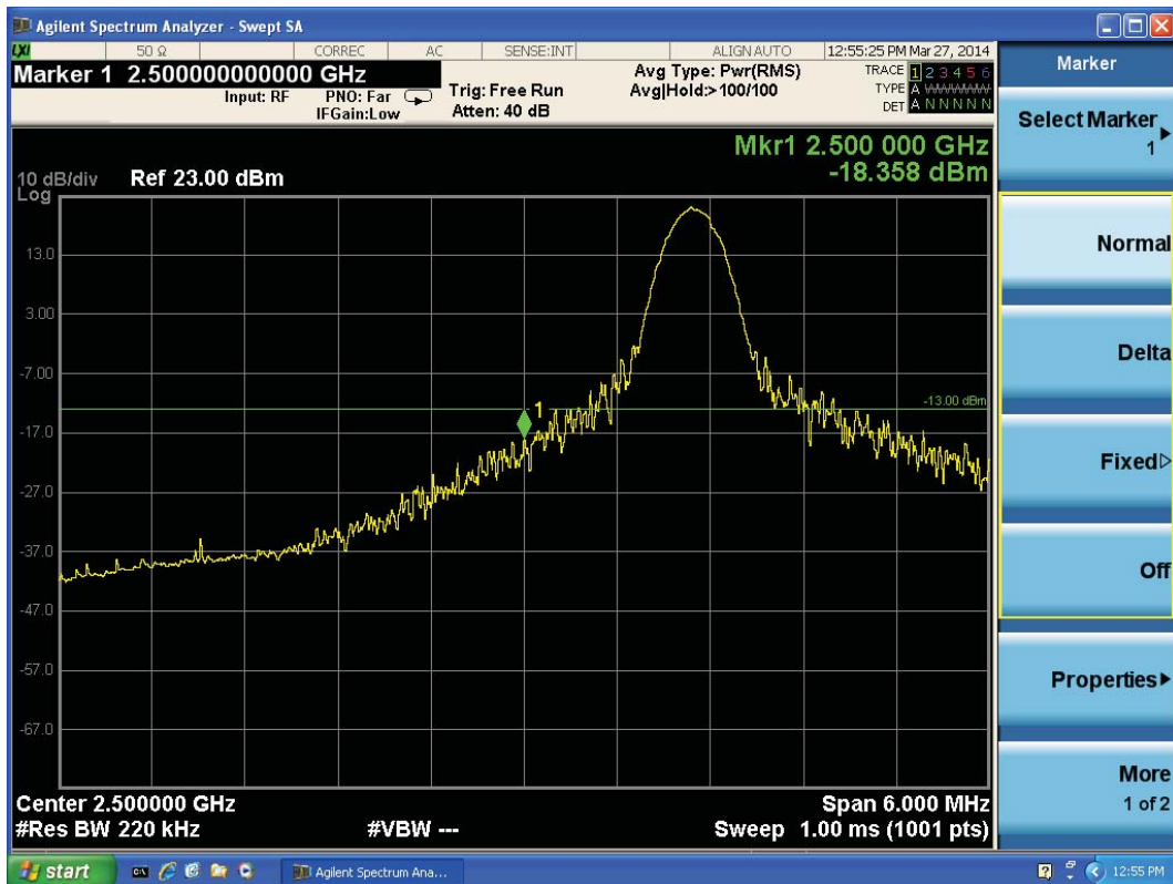
LTE Band 7 16QAM Bandwidth = 20MHz CH20850, RB 1
