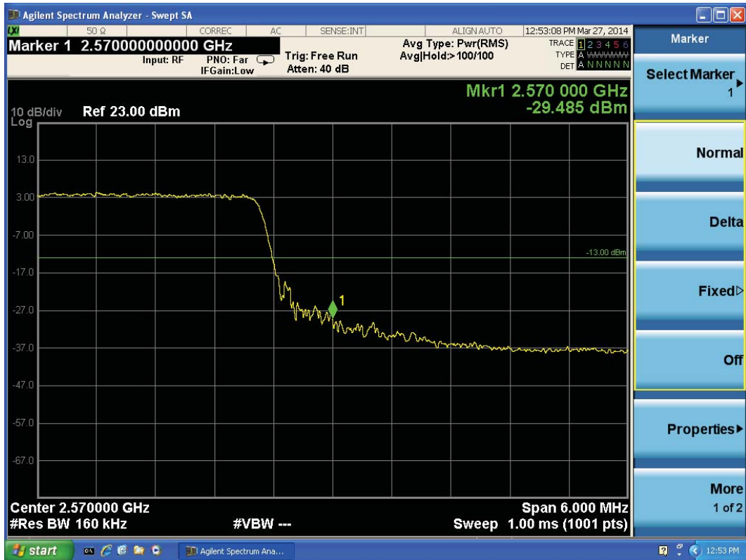
LTE Band 7 16QAM Bandwidth = 15MHz CH21375, RB 38
