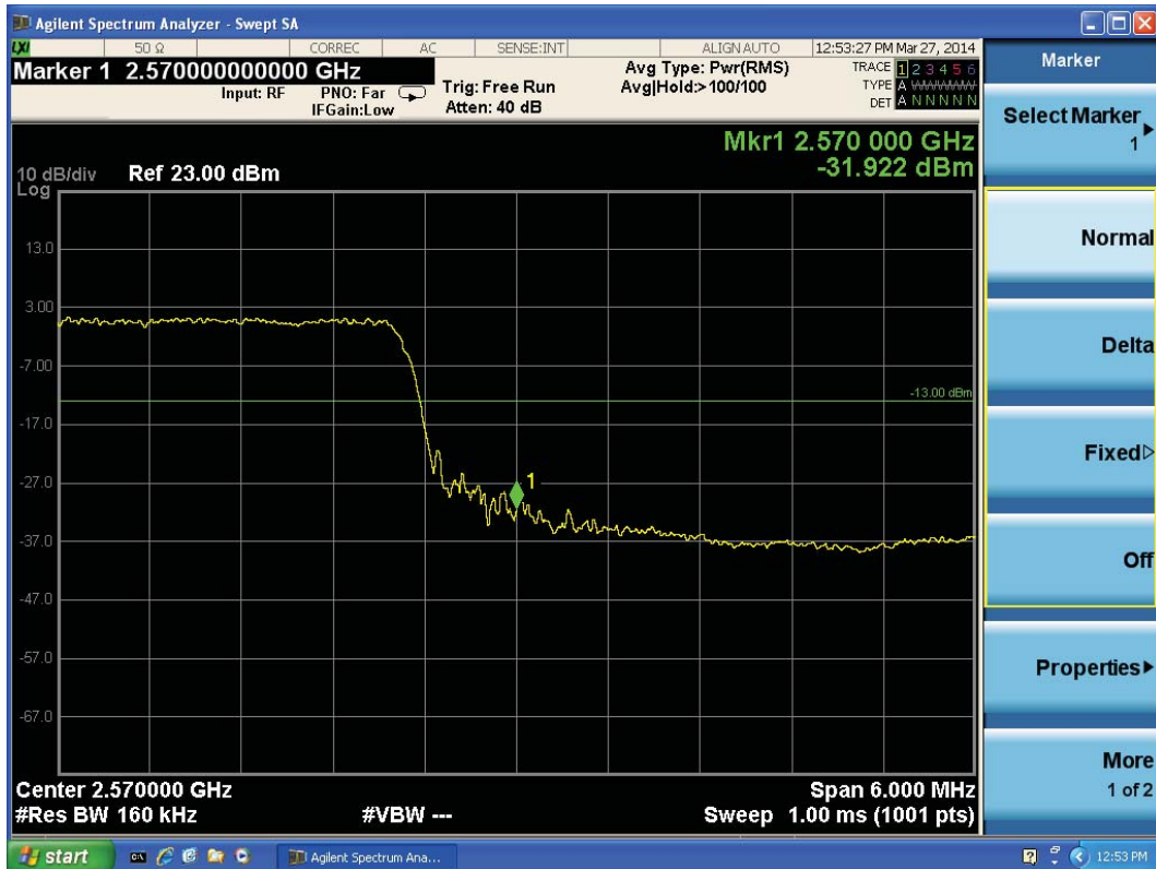
LTE Band 7 QPSK Bandwidth = 15MHz CH21375, RB 75
