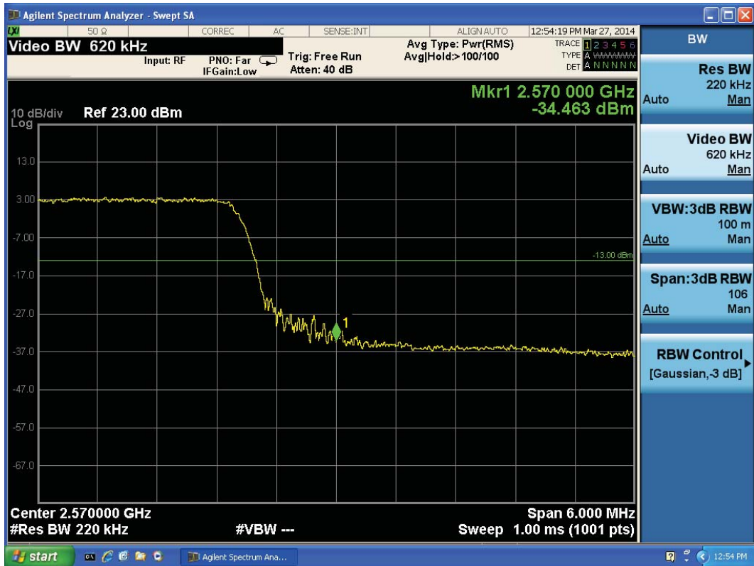
LTE Band 7 16QAM Bandwidth = 20MHz CH21350,RB 50
