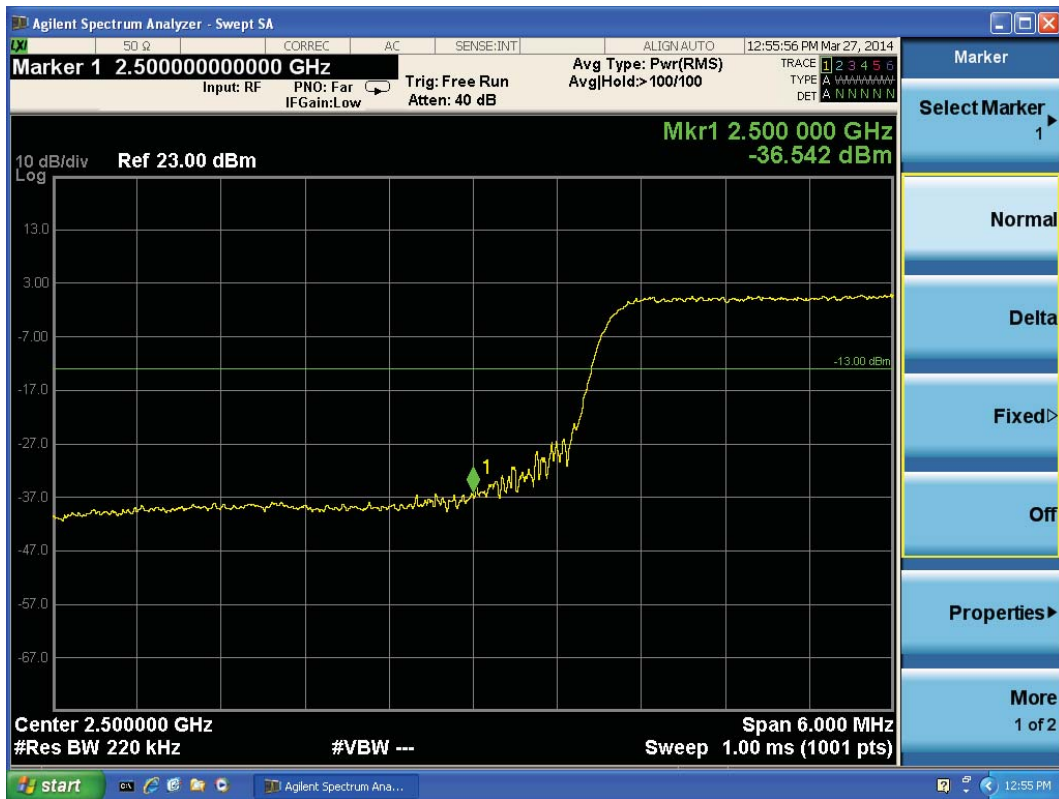
LTE Band 7 16QAM Bandwidth = 20MHz CH20850, RB 100
