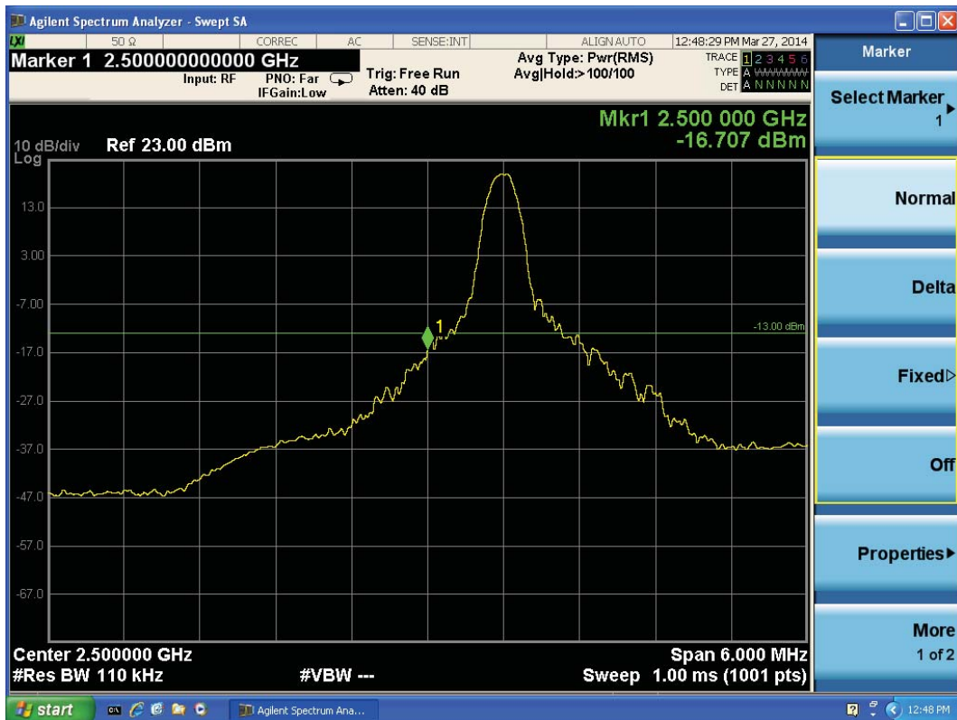
LTE Band 7 16QAM Bandwidth = 10MHz CH20800, RB 1
