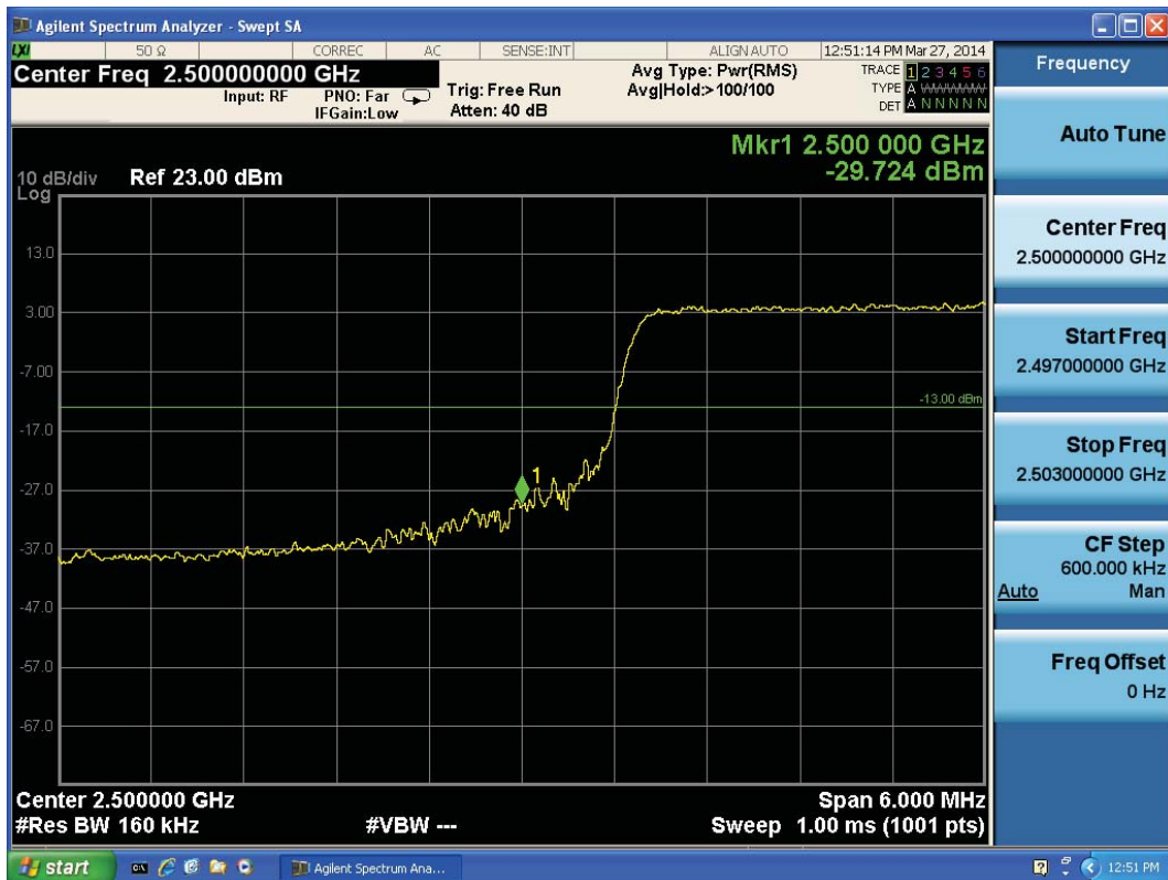
LTE Band 7 16QAM Bandwidth = 15MHz CH20825, RB 38
