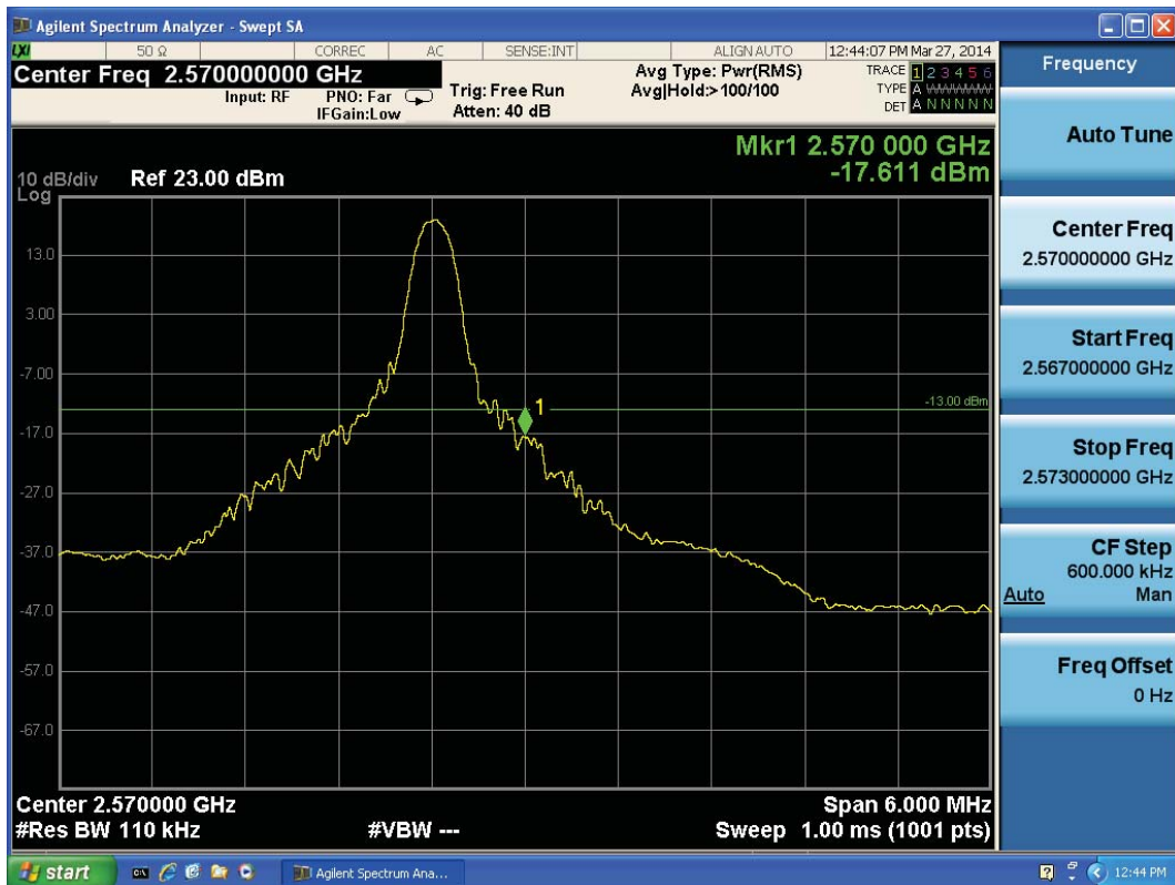
LTE Band 7 16QAM Bandwidth = 10MHz CH21400, RB 1
