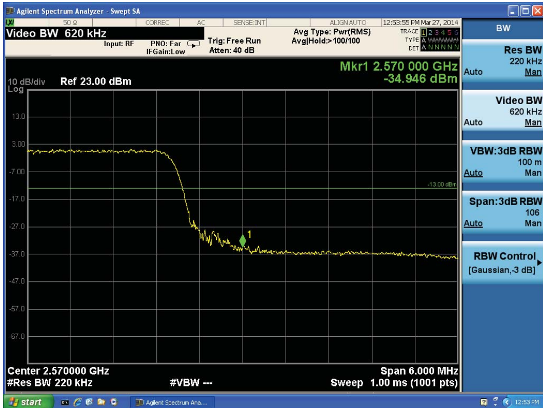
LTE Band 7 QPSK Bandwidth = 20MHz CH21350, RB 100
