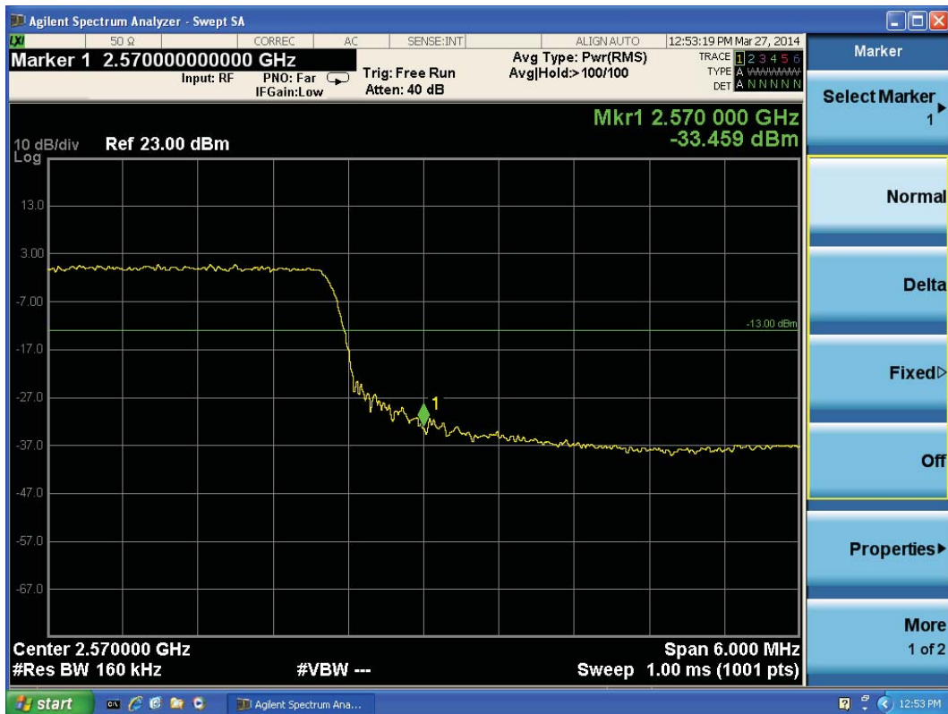
LTE Band 7 16QAM Bandwidth = 15MHz CH21375, RB 75
