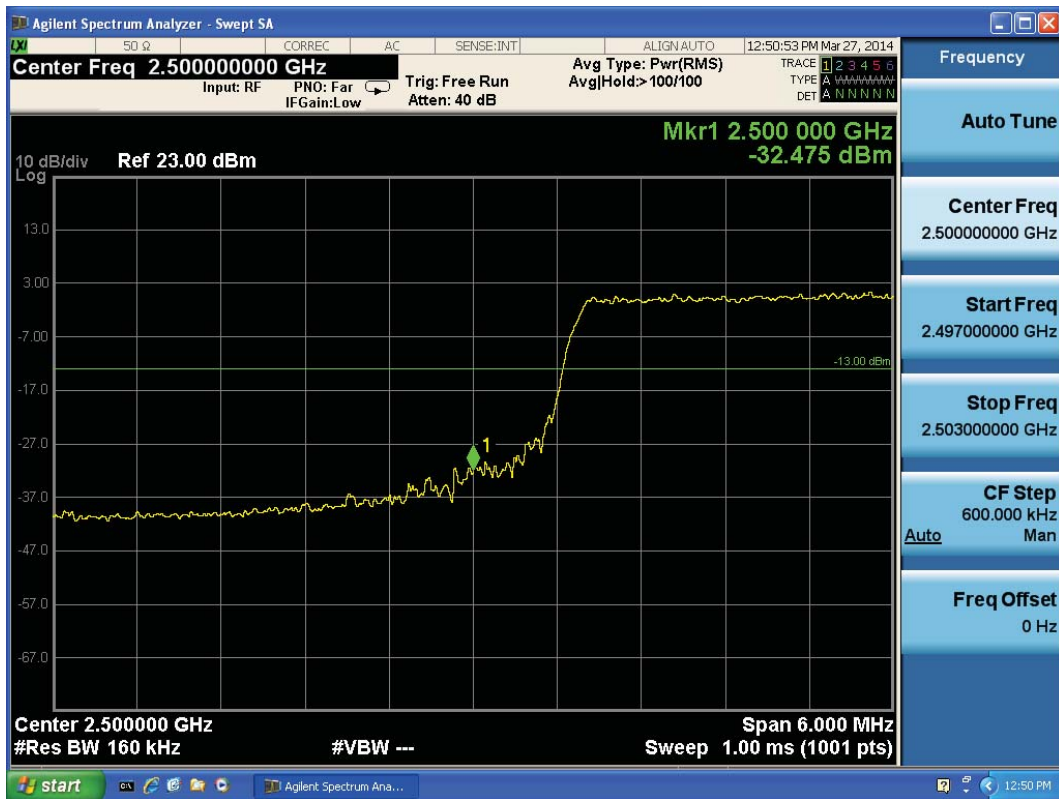
LTE Band 7 16QAM Bandwidth = 15MHz CH20825, RB 75
