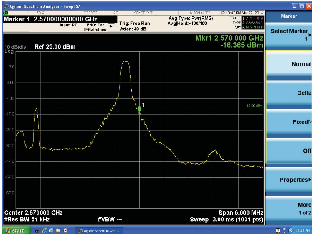
LTE Band 7 16QAM Bandwidth = 5MHz CH 21425, RB 1
