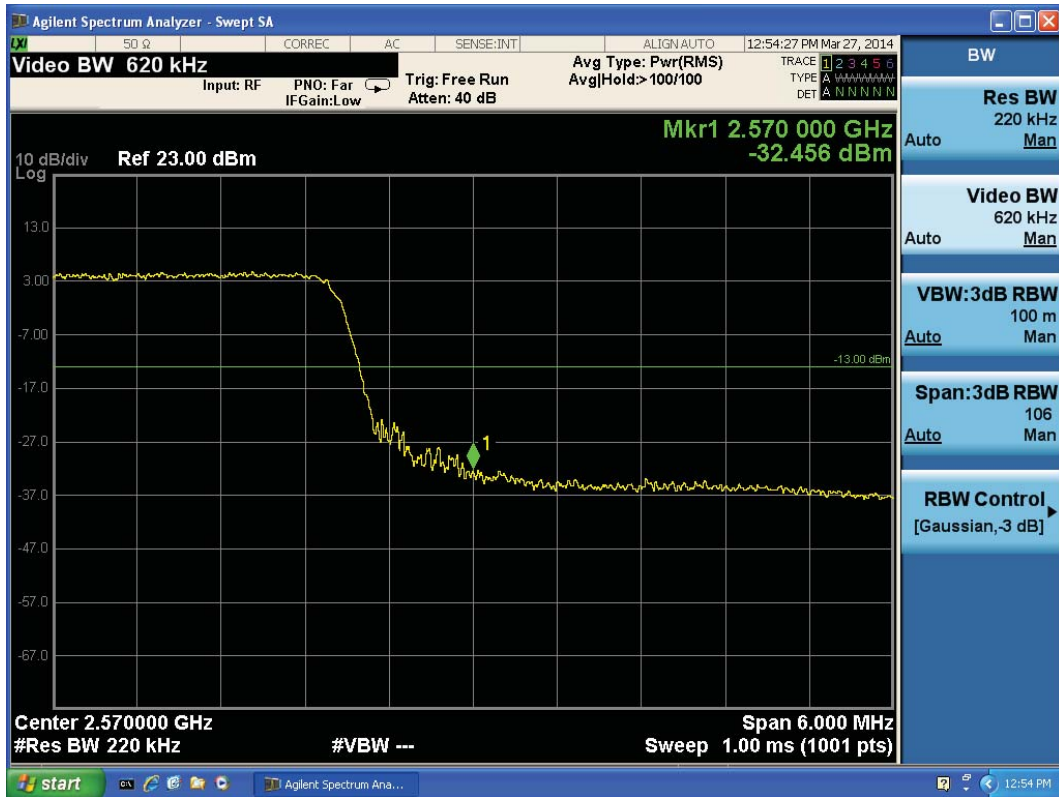
LTE Band 7 QPSK Bandwidth = 20MHz CH21350, RB 50
