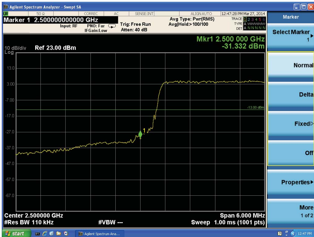
LTE Band 7 16QAM Bandwidth = 10MHz CH20800, RB 25
