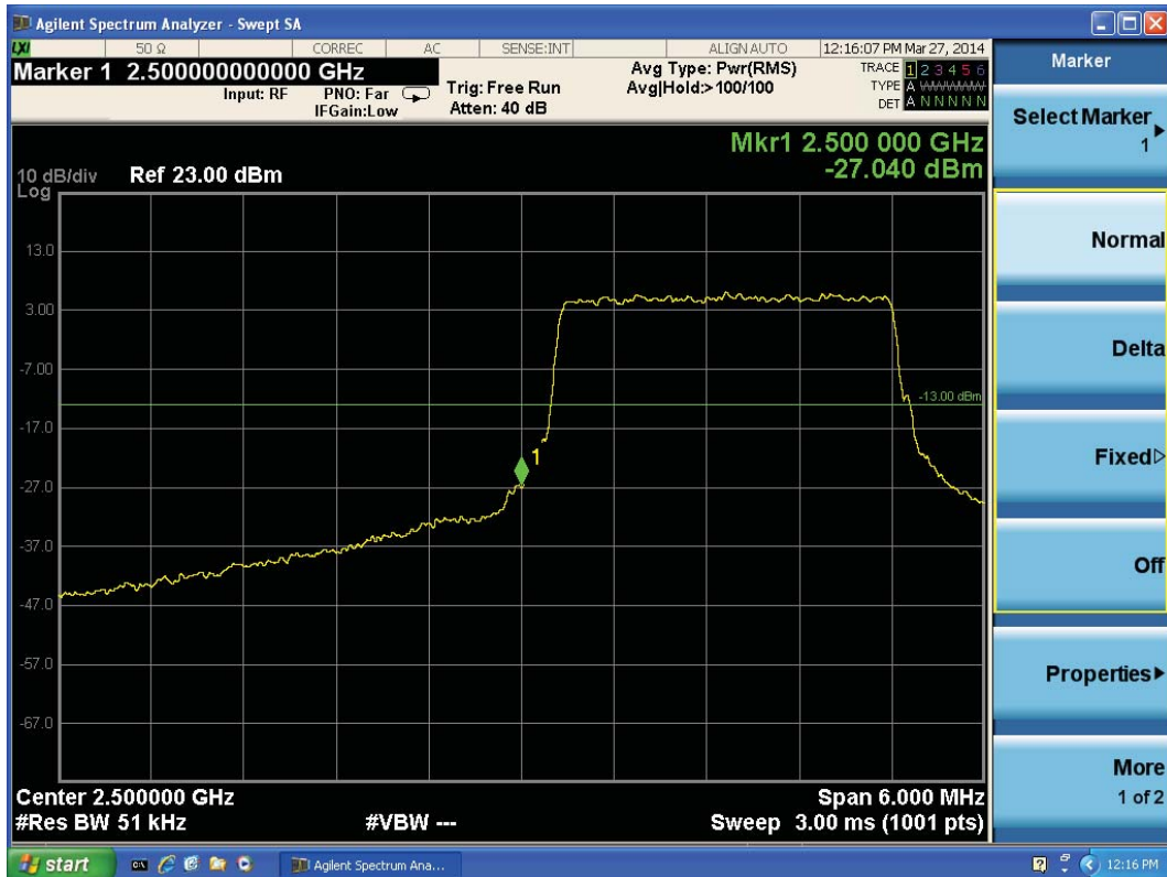
LTE Band 7 16QAM Bandwidth = 5MHz CH 20775, RB 12
