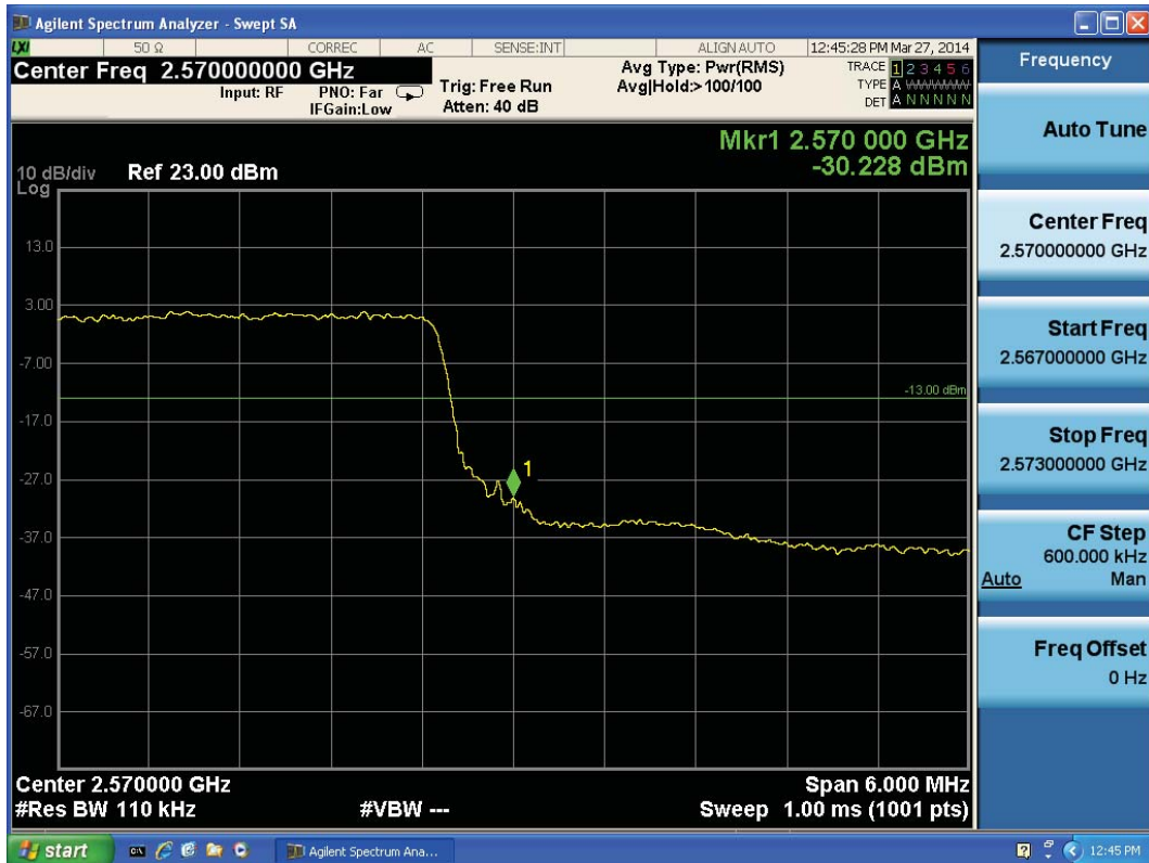
LTE Band 7 16QAM Bandwidth = 10MHz CH21400, RB 50
