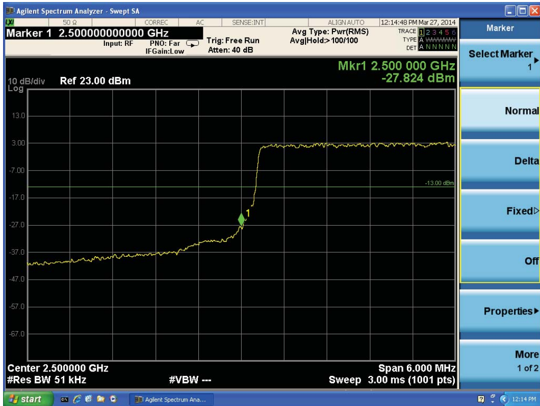
LTE Band 7 16QAM Bandwidth = 5MHz CH 20775, RB 25
