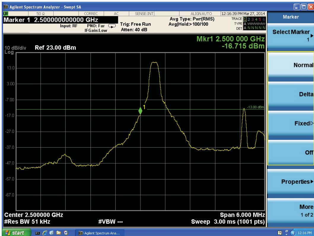
LTE Band 7 16QAM Bandwidth = 5MHz CH 20775, RB 1
