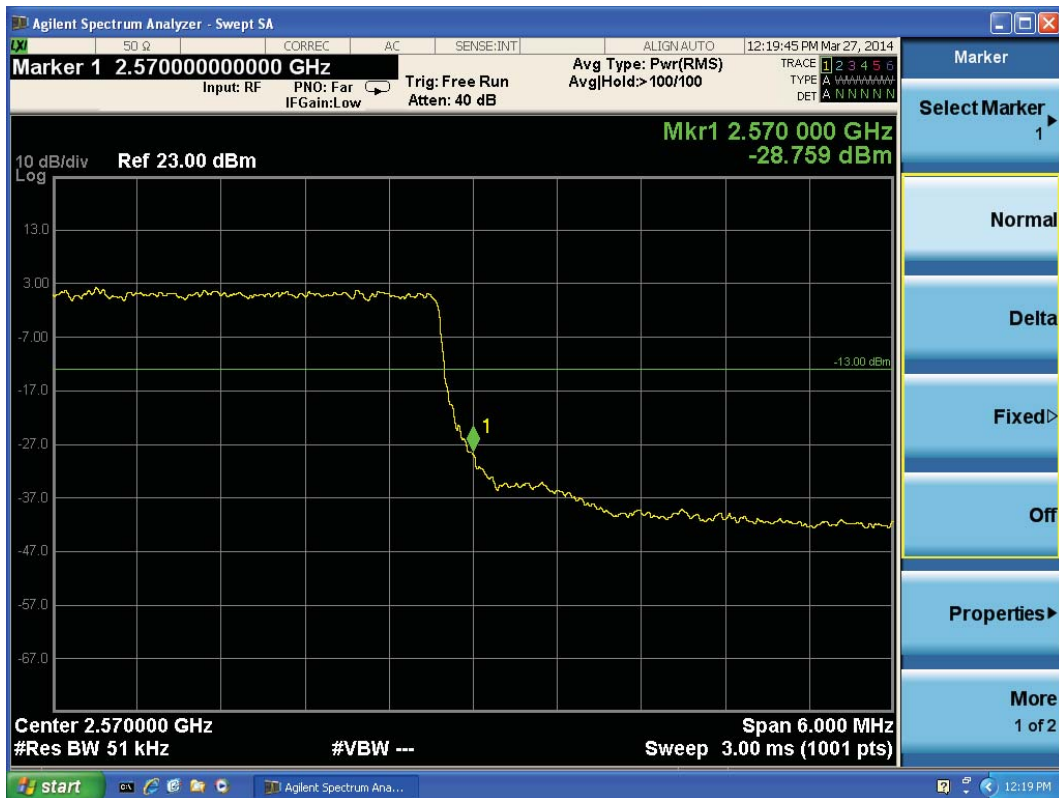
LTE Band 7 16QAM Bandwidth = 5MHz CH 21425, RB 25
