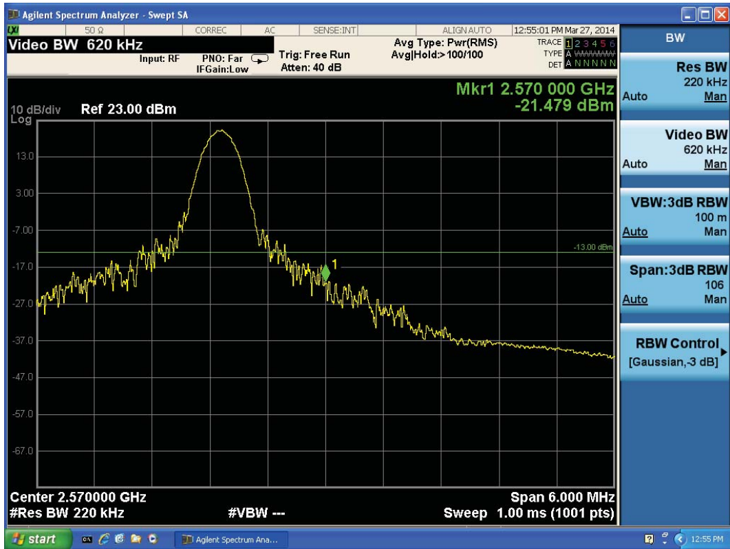
LTE Band 7 16QAM Bandwidth = 20MHz CH21350,RB 1
