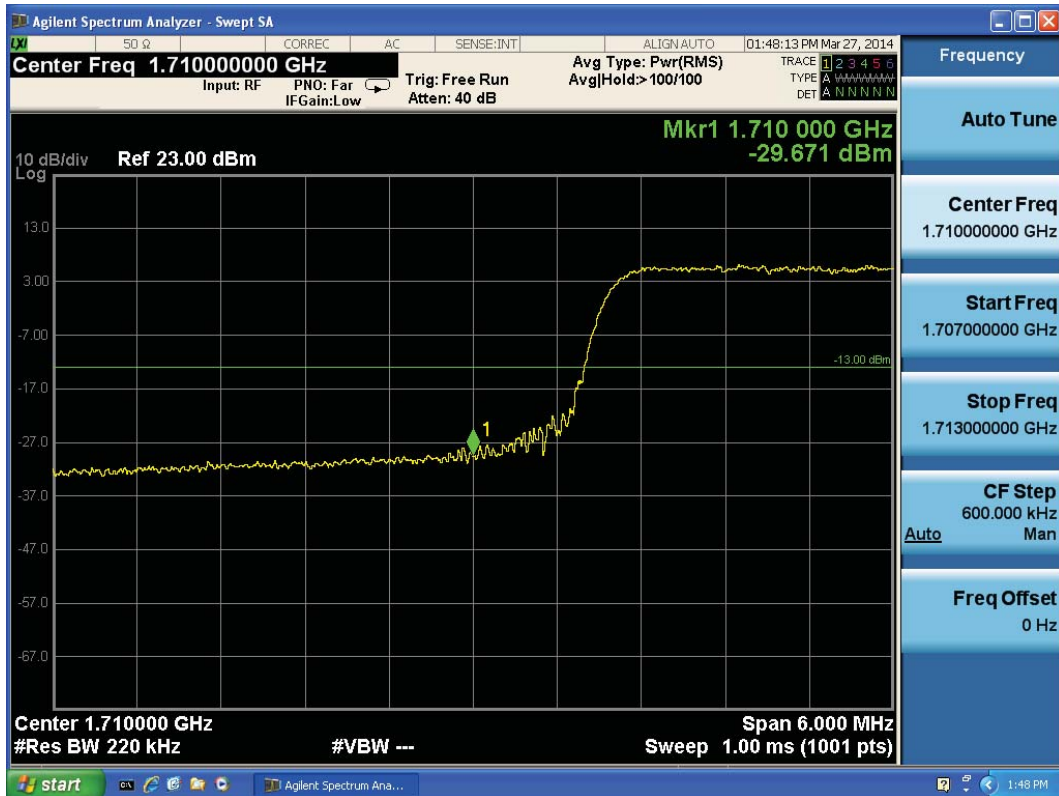
LTE Band 4 16QAM Bandwidth = 20MHz CH20050, RB 50
