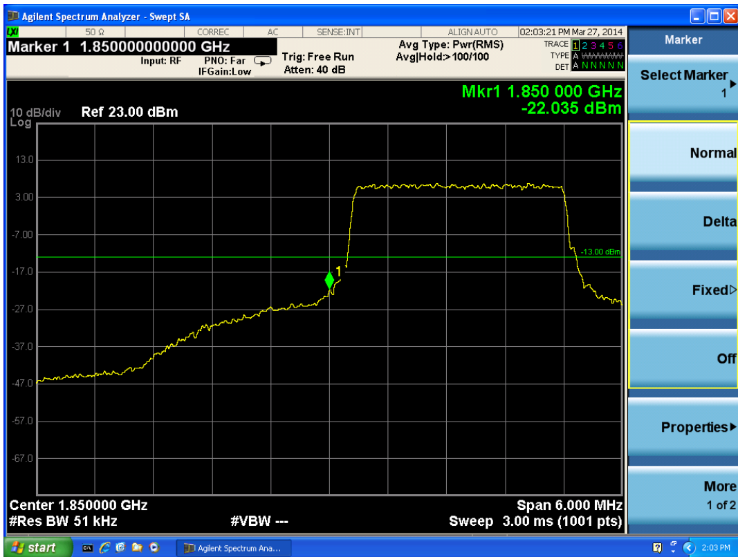
LTE Band 2 16QAM Bandwidth = 5MHz CH18625, RB 12
