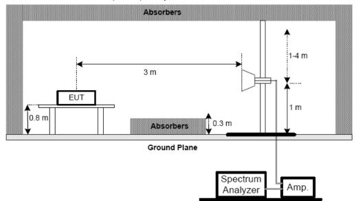
Note: The antenna can be moved between 1 to 4 meters above the ground.
