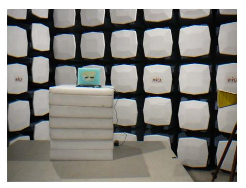
14.2 Radiated Emissions below 1 GHz - Rear View
