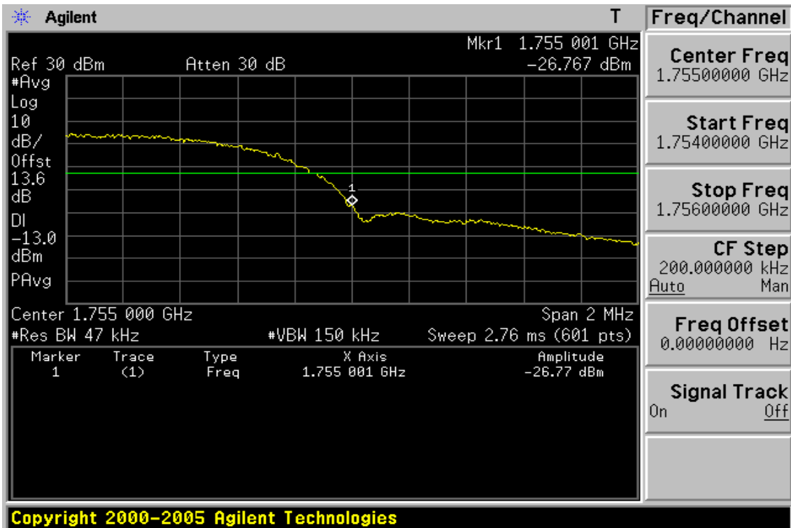
Figure 9-15: Band edge emission at antenna terminals –HSUPA IV Channel Highest
