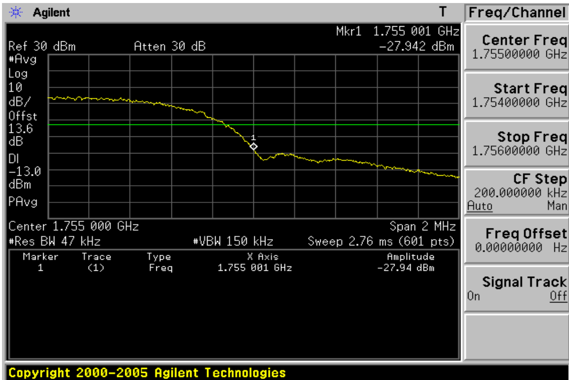
Figure 9-5: Band edge emission at antenna terminals – WCDMA IV Channel Highest
