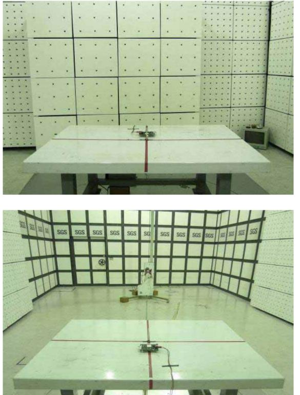
Radiated Emission Set up Photos (E2 Mode)
