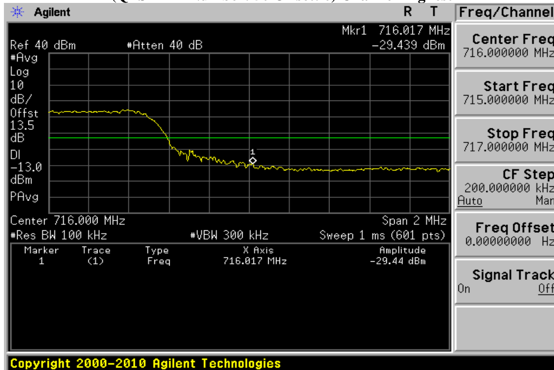
Figure 10-270: Band edge emission at antenna terminals –10MHz BW LTE-Band 17 (QPSK RB Number: 50 Offset: 0) Channel Highest
