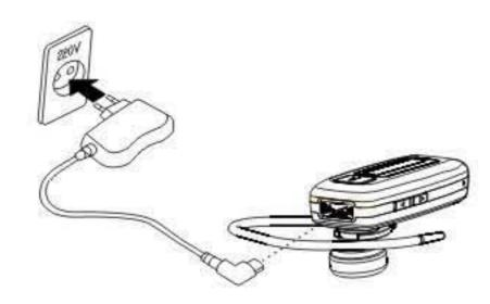
2. Plug the travel adapter into the case's charging socket.
