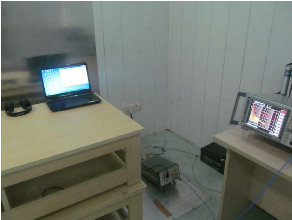
FCC RADIATED EMISSION TEST SETUP
