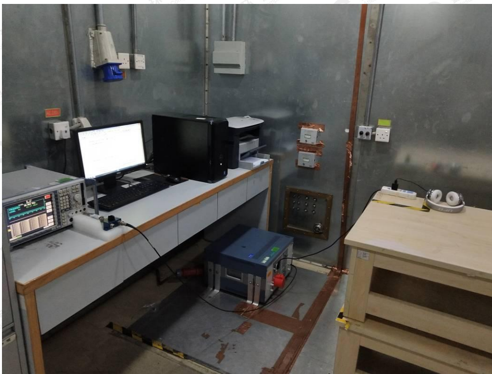
FCC RADIATED EMISSION TEST SETUP
