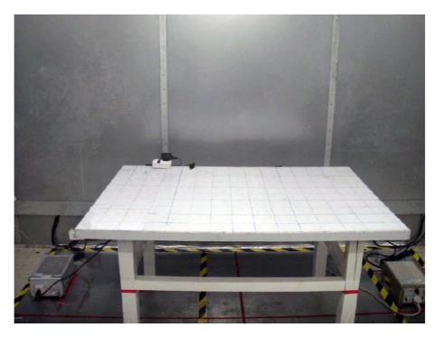
RADIATED EMISSION TEST SETUP
