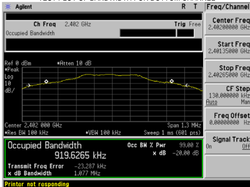
TEST PLOT OF BANDWIDTH FOR BOTTOM CHANNEL
