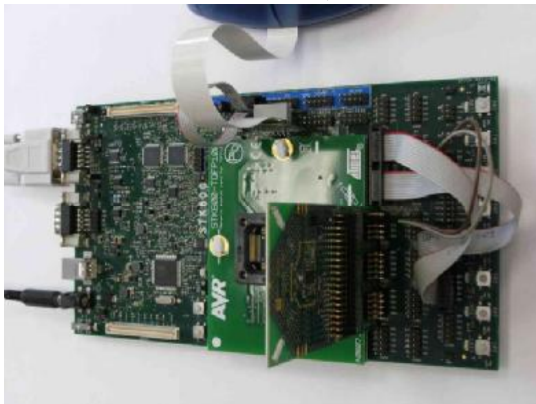
Figure 10-19. STK600 (with ATxmega128A1) with REB to STK600 Adapter and REB connected to JTAG-ICE and UART, and LED and Button Cable
